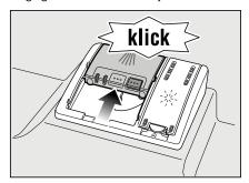
The detergent dispenser opens automatically at the optimum time depending on the programme. The powder or liquid detergent is distributed in the appliance and is dissolved, the tablet falls into the tablet collecting tray where it dissolves in doses.
