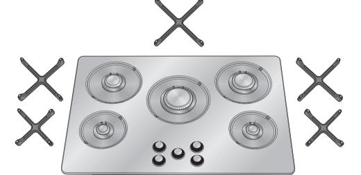
Each rack must be positioned on the corresponding burner in order to guarantee proper operation. Be very careful to match the different central diameters of the racks to the flame-spreader crowns.
