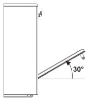
To reassemble the door, put the hinges in the relevant slots in the oven, making sure that grooved sections **C** are resting completely in the slots. Lower the door and once it is in place remove the pins from the holes in the hinges.
