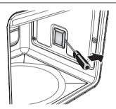
Remove the bulb by unscrewing (filament bulbs) or pulling it out (halogen bulbs) in the indicated direction. Replace the bulb with one of the same type (25W for filament bulbs or 40W for halogen bulbs).
