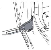
Grasp the door on both sides with both hands, lift it forming an angle of around 30° and remove it.
