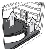
Lift up the edge of the lower heating element a few centimetres and clean the bottom.
