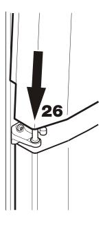
**19.** Transfer the hinge component on the hinge bracket to the opposite side.
