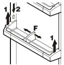
Place the shelf rails provided, fig. 1, on the supports on the left and right at the desired height.
