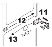
**24.** Suspend bottom door on hinge pin and close.
