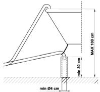
The free end should be positioned at a height of between **30 and 100 cm**, and should never be submerged in water. If a horizontal drain extension hose is used (for a maximum of 3 m) the drain hose can be placed at a maximum height of **85 cm** from the ground.
