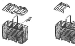
The cutlery basket slides across the dishwasher and can be **placed in** any position to allow optimal use of the space in the bottom basket.
