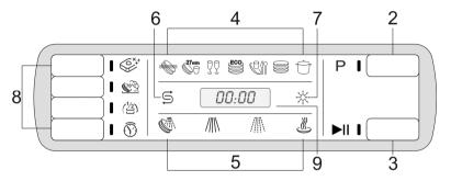
The light of the phase in progress will flash, while the lights of the subsequent phases remain on.
