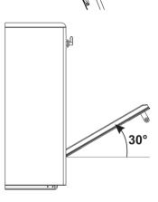
To reassemble the door, put the hinges in the relevant slots in the oven, making sure that grooved sections C are resting completely in the slots. Lower the door and once it is in place remove the pins from the holes in the hinges.
