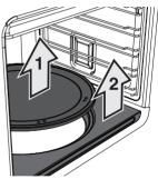
Lift up the edge of the lower heating element a few centimetres and clean the bottom.
