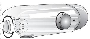
that has the same characteristics (E14,  $\max$  15 W), screwing it back in the opposite direction to that shown in the figure.
