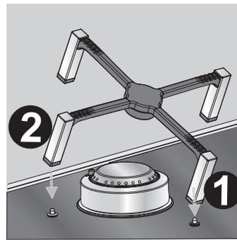
To position the rack, you first need to centre the fastening pins (1) and (2) and then lower it until it is resting on the hob. When properly positioned, the legs of the racks must not be suspended above the hob but should rest on top of it.
