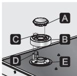
The burner caps and flame diffuser rings can be removed for easier cleaning; wash them in hot water and non-abrasive detergent, taking care to remove all deposits, and wait for them to **dry completely**.
