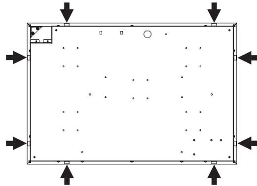
To fit the clips to the hob, simply press them gently horizontally into the groove provided (**fig. A**). Then turn them upwards to fix them permanently in place (**fig. B**).
