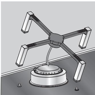
Each rack must be positioned on the corresponding burner in order to guarantee proper operation. Be very careful to match the different central diameters of the racks to the flame-spreader crowns.
