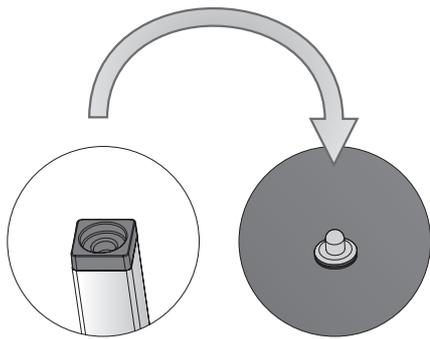
At the ends of the legs of the racks there are silicone rests with a hole that must be centred onto the matching fixing pins on the hob.
