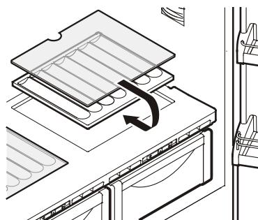
Remove the glass plate and insert it under the shelf plate.
