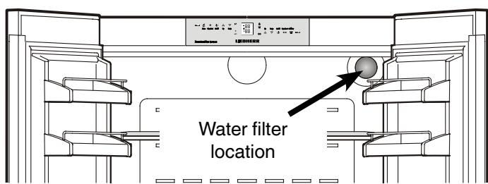
Replace the filter when the waterdrop symbol appears in the temperature display.
