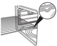
To remove the rack or tray, lift the front slightly.
