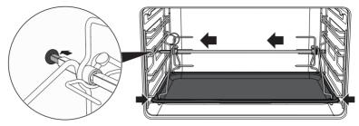
At the end of cooking, screw on the handle provided so that you can move the rod with the food on it readily.
