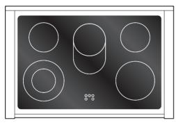
The appliance has 5 cooking zones of various diameters and power levels. Their position is clearly indicated with circles and heat is released within the diameters traced on the glass ceramic surface. The 5 cooking zones are HIGH-LIGHT zones and come on a few seconds after activation. The heat intensity can be adjusted using
