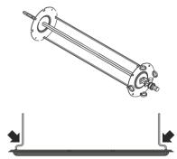
Place the rotisserie rod on the supports. Make sure the pins are correctly positioned on the shaped part of the supports.
