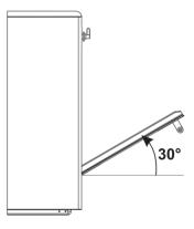
To reassemble the door, put the hinges in the relevant slots in the oven, making sure that grooved sections C are resting completely in the slots. Lower the door and once it is in place remove the pins from the holes in the hinges.
