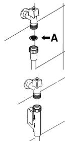
The dishwasher can also be connected to a hot water supply **not exceeding 60°C**. Supplying the appliance with hot water cuts down the washing time by approximately 20 minutes, but slightly reduces its effectiveness. Make the connection to the domestic hot water supply using the same procedure described for connecting to the cold water supply.
