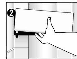
Hold the bottom of the light cover and pull forward to remove.
