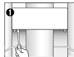
Remove the 2 screws retaining the light cover.
