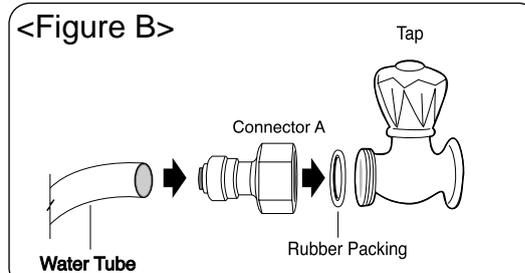
**N.B.** Place the rubber washer inside the tap connector and screw onto the water tap.
