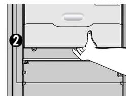
Hold the bottom of cover and pull forward to remove.
