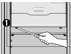
Remove the screws retaining the light cover.
