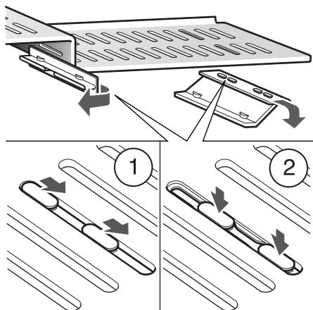
If a different size of Gastronorm drawer is to be used, the positions of the holders can be changed.
