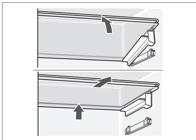
Before the extendable glass shelf can be removed, the serving tray must be removed.
