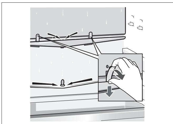
Regularly clean condensation channels and drainage hole with cotton buds, etc. so that the condensation can run out. The upper condensation channel can be taken out for cleaning.
