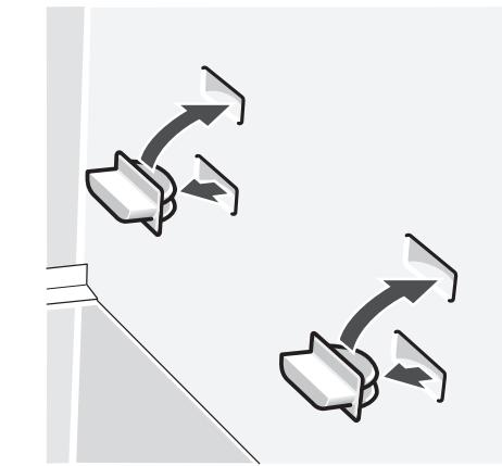
The position of the glass shelf can be changed by moving the stoppers.
