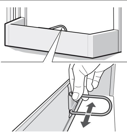
The bottle holder prevents bottles from falling over when the door is opened and closed.
