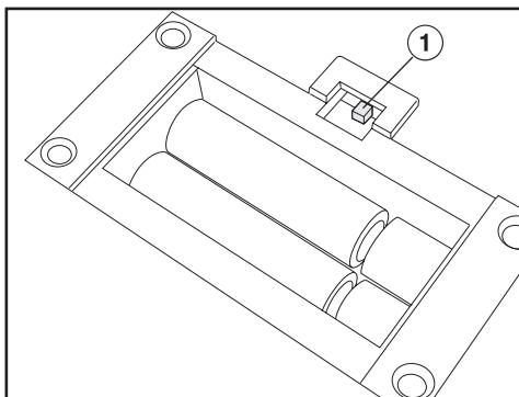
The switch ① for changing from metric to imperial measurements is located in the battery compartment.
