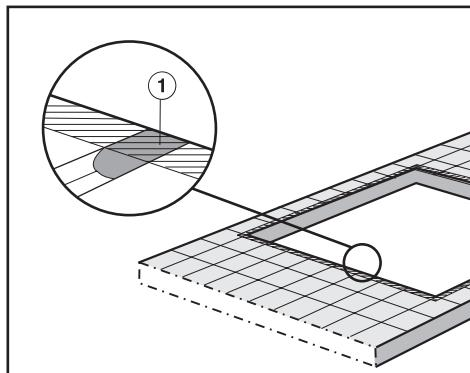
Grout lines ① and the hatched area underneath the surface of the appliance must be smooth and even. If they are not, the appliance will not sit flush with the worktop and the sealing strip underneath the top part of the appliance will not provide a good seal between the appliance and the worktop.
