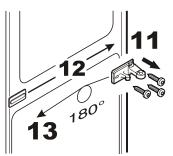
**24.** Suspend lower door on hinge pin and close
