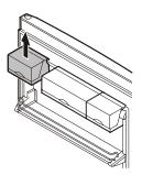
To detach the lid: open 90° and raise to disengage.
