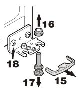
**26.** Suspend upper door on hinge pin and close.
