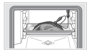
If there are several pieces, insert the core temperature probe in the middle of the thickest piece.
