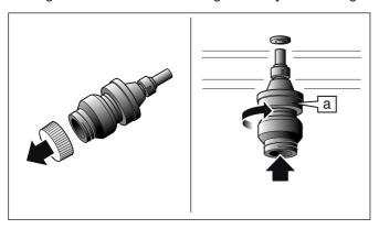
6 Screw the cleaning cartridge (a) fully into the socket in the top of the cooking compartment. Close the appliance door. Press ✓ to confirm. A cleaning time of 3 hours 45 minutes will be displayed.
