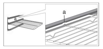
When pushing in the perforated cooking container, make sure that the recess (a) is pointing to the side.
