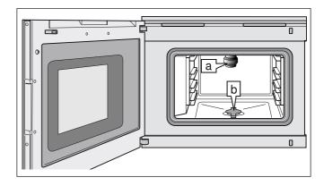
The cleaning programme removes stubborn dirt.A cleaning cartridge (a) is screwed into the top of the cooking compartment. The cooking compartment is cleaned, rinsed and dried fully automatically. The drain filter (b) must remain inserted in the cooking compartment floor while the cleaning programme is in progress.
