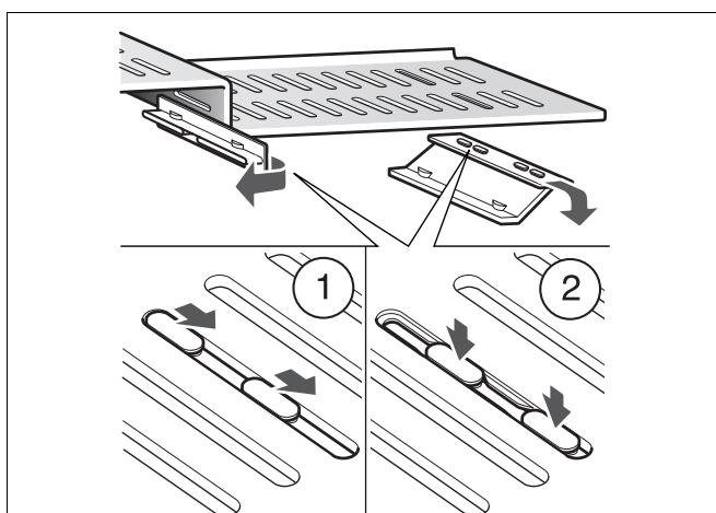
If a different size of Gastronorm drawer is to be used, the positions of the holders can be changed.
