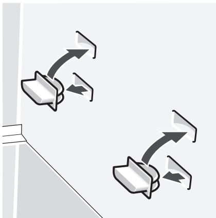
The position of the glass shelf can be changed by moving the stoppers.
