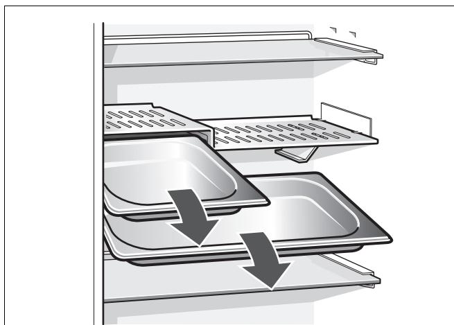
Food can be stored in the Gastronorm drawer and placed in the refrigerator compartment with minimum space requirements.
