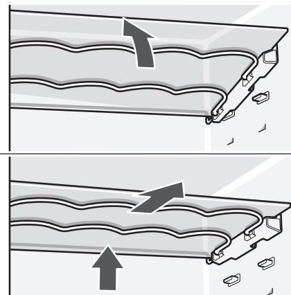
To remove the glass shelf, pull up at an angle and take out.
