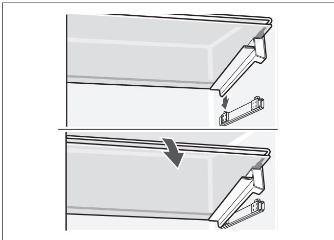
Fit back of glass shelf, position and engage by pressing down the front of the shelf.
