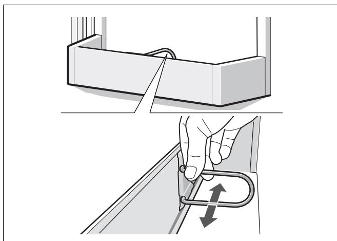
The bottle holder prevents bottles from falling over when the door is opened and closed.
