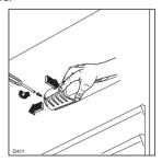
If the door is open and the light does not come on, check that the bulb is properly screwed in; if it still does not work, replace the bulb with one of the same power
