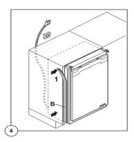
4. The joint cover (B) is to be assembled after having installed the appliance in the recess.
