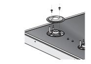
Remove the hob skin fixing screws, taking care only to remove the screws shown on the right.
